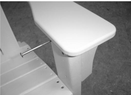
Arms should be installed with curve side on the inside of the chair (Left Picture). Place Arm on top of Front Leg. Align pre-drilled hole in arm with the pre-drilled hole located at the top of the Front Leg. Install a 3-1/2" connector bolt through pre-drilled hole in Front Leg, then through pre-drilled hole under arm. Install flat washer, lock washer, and nut. Do not tighten at this time. Repeat process on other side.
