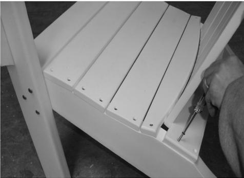
Place Seat Assembly on top of mounting surface of Rear Legs (Left Picture). Push Back Assembly forward until it's aligned with Seat Assembly. Hold Back Assembly in place and install (4) 1-3/4" Phillip's Head Screws into pre-drilled holes on each side.
